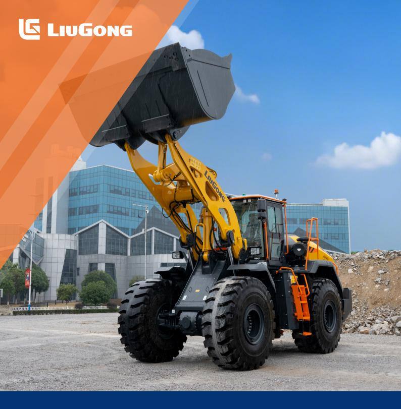
EngineCummins X12Max. Gross287 kW (385 hp / 390 ps) @ 1,800 rpmMax. Net273 kW (366 hp / 371 ps) @ 1,800 rpmOperating Weight31,750 kgStandard Bucket Size5.4 m³Standard Breakout Force270 kNStandard Dump Clearance3,332 mm
